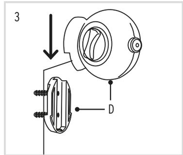
4. **Drill two suitable holes in the opposite location, then plug with (A) and screw in the detachable bracket from the hook (C), using two screws (B). Slide hook over fixed bracket.**
