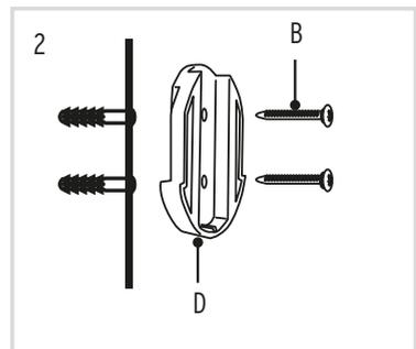
3. **Attach the retractable line case to the fixed bracket.**
