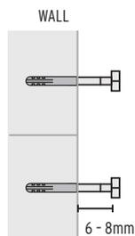
6. Align and locate cabinet mounting hole into screw and pull down slightly to secure correctly. Tighten screws into positions.
