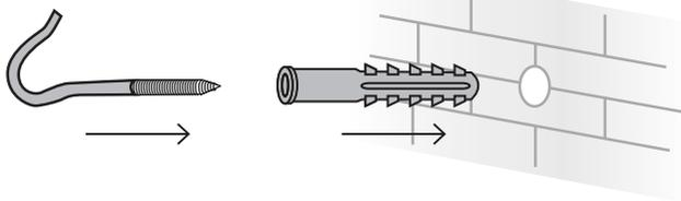
5. To install cabinet, insert plastic plug into the hole and affix screws leaving 6-8mm distance from shoulder head to the wall.
