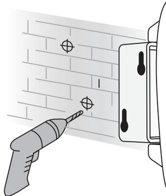
3. In retaining hook wall side, drill hook position with 8mm diameter x 35 - 40mm depth. (For Twin Line model, repeat Step 3 to drill second hook position. Recommended centre to centre hole positions 50mm - 80mm.)
