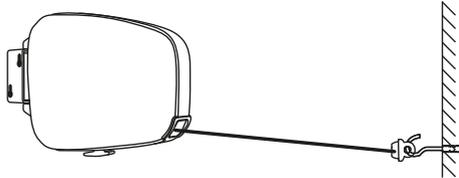
3. From cabinet side, pull the line taut and loop around safety anchors twice to secure the line. (For Twin Line model, repeat Step 1 - 3 to extend second line)
