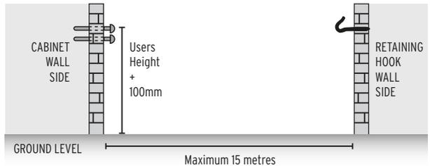
2. In cabinet wall side, turn mounting bracket facing against the wall and mark two hole positions.
