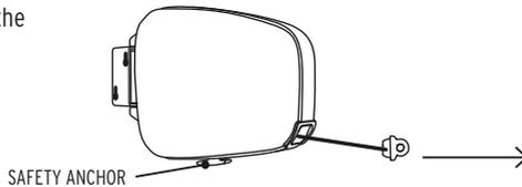
2. Extend line and securely hook onto the retaining hook on the opposite wall.
